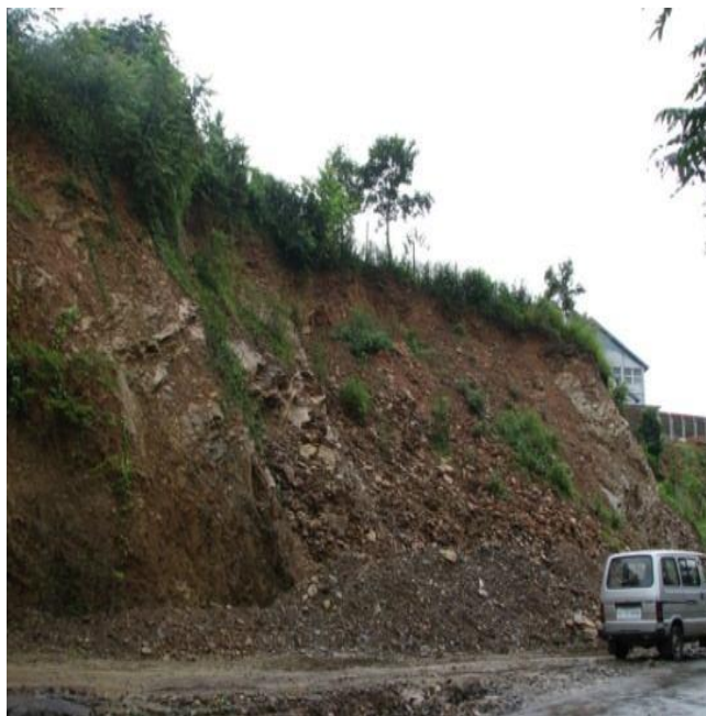
Figure 2. Debris slide in sheared rocks
