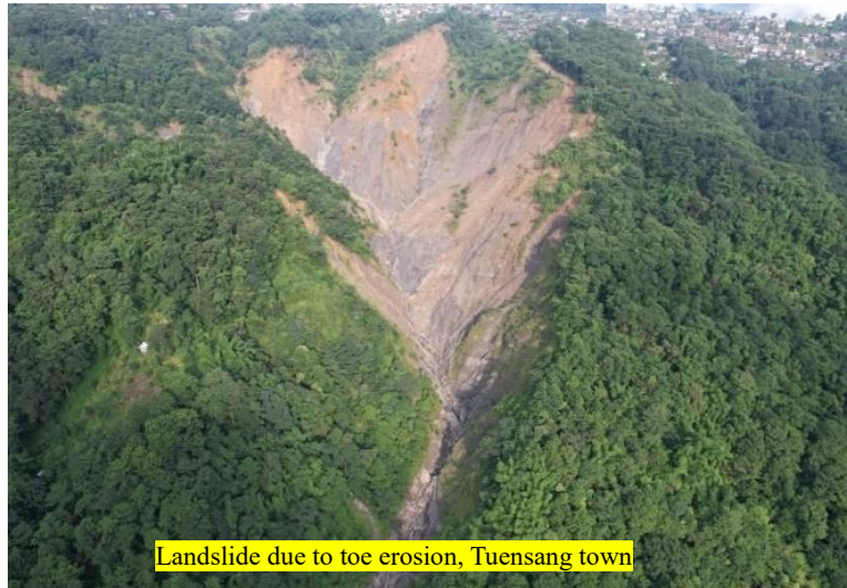
Landslide due to toe erosion, Chathi river
